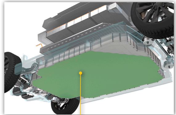
Pack Tray Corrosion & Impact Protection
