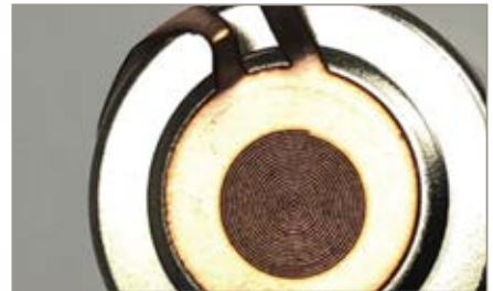
Spiral welding battery tab
