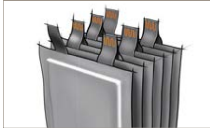
Weld pouch cell tabs
