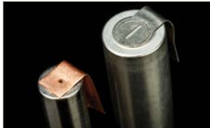
Dissimilar metal welding
