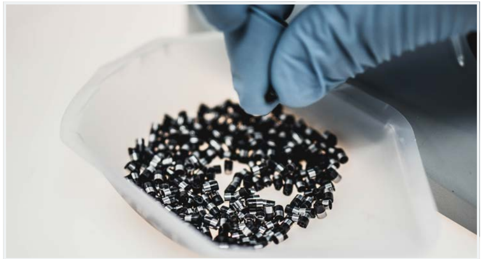
The tip design required extreme micro tooling precision to accomplish the tiny through-holes required for this application. Extremely thin walls in this overmolded tip design measuring .005" at the overmolded section of the metal ring and features +/- .001" tolerances throughout were enabled by micro injection molding technology.
